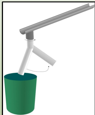
Rotating piping allows the rainwater to be channelled to the receptacle only when you want it.
